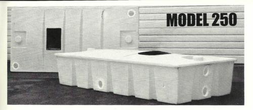
**MODEL 250** comes complete with seven 3" fittings and plugs, giving the option of hooking into a series to expand holding capacity. Two 4" C.I.T. nipples and a removable inspection port are included. Unit is designed to be used above ground only.
