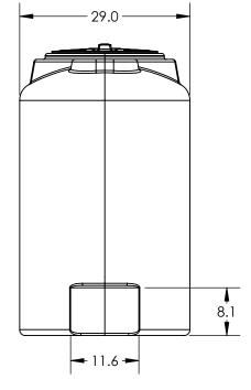
\*ALL EXTERNAL PIPING MUST BE INDEPENDENTLY SUPPORTED. \*ONLY BASE FITTINGS TO BE LEFT INSTALLED AT TIME OF SHIPMENT PER SII PROCEDURE. ALL DIMENSIONS ARE IN INCHES, NOMINAL, & SUBJECT TO CHANGE WITHOUT NOTICE. ALL DIMENSIONS ON ROTATIONAL MOLDED PARTS ARE SUBJECT TO A  $\pm$  3% TOLERANCE.
